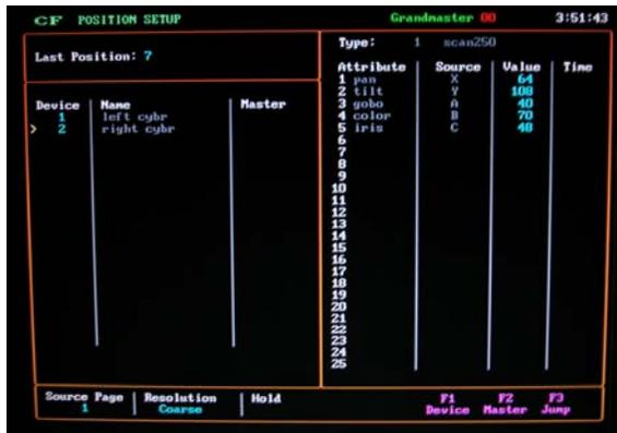
Figure 87– Position Setup Screen
