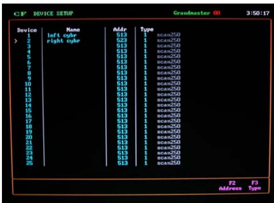
Figure 86-Device Setup Screen with start addresses assigned
